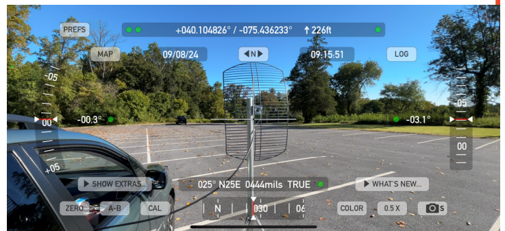
wideband grid parabolic aiming with Theodolite phone app
